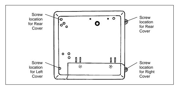
Figure 5-2 Left/Right Bottom Screw Location
